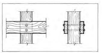
Figure 4.31. Bolted Connection to Round Pole
