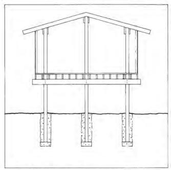
Figure 4.29. Pole Frame Construction
