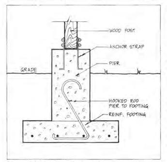
Figure 4.9. Post/Pier Foundation
