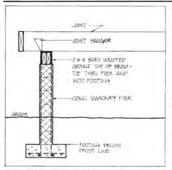
Figure 4.35. Concrete Masonry Unit Pier
