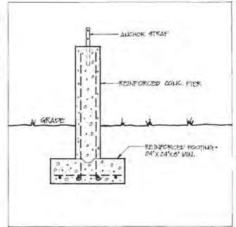
Figure 4,19. Reinforced Concrete Pier
