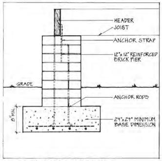
Figure 4.16. Reinforced Brick Pier
