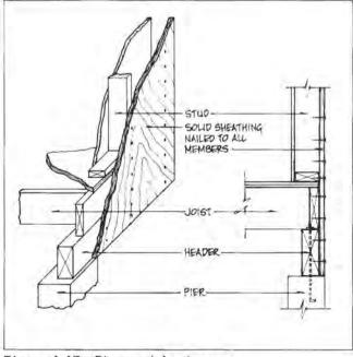
Figure 4.45. Plywood Anchorage
