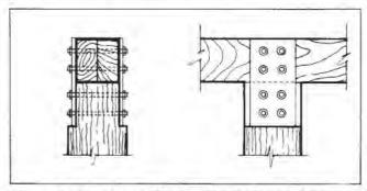
Figure 4.32. Dapped Gusset Plate Connection
