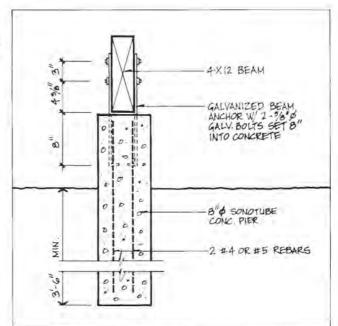
Figure 4.20. Drilled Pier Foundation
