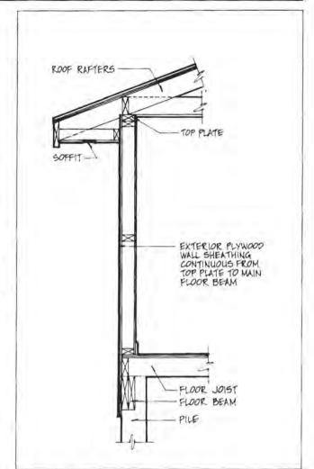
Figure 4.46. Wall Sheathing Tie from Roof to Ceiling
