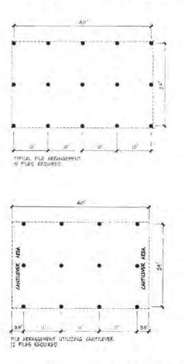
Figure 4.40. Cantilever Used to Reduce Number of Foundation Elements
