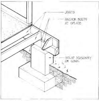
Figure 4.38. Beam Splice on Pier
