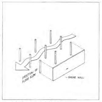
Figure 4.24. Shear Wall Bracing
