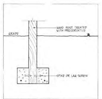
Figure 4.11. Spike Anchorage of Post
