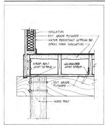
Figure 4.51. Insulated Floor Section, Wood Post Foundation
