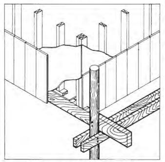
Figure 4.30. Exterior Pole Framing
