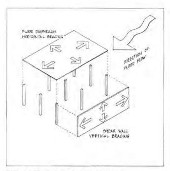
Figure 4.25. Floor Diaphragm Bracing
