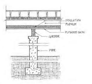
Figure 4.53. Double-Insulated Floor Plenum, Pier Foundation
