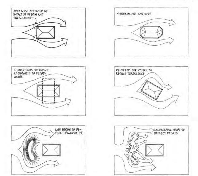
Figure 2.6. Site Design to Reduce Flood Hazards
