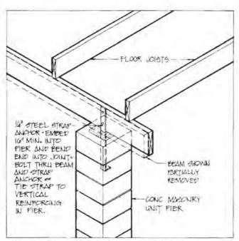
Figure 4.36. Masonry Pier-Strap Anchor
