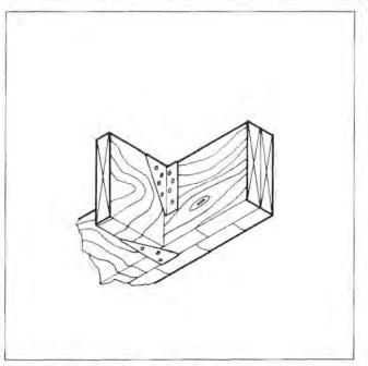
Figure 4.27. Metal Framing Anchors
