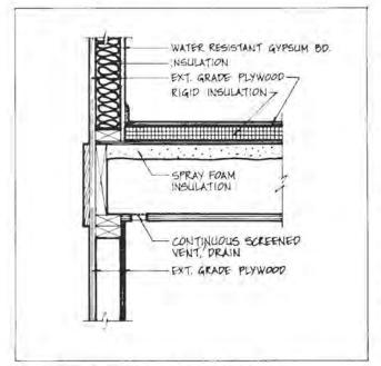
Figure 4.52. Insulated Floor Section, Foundation Wall
