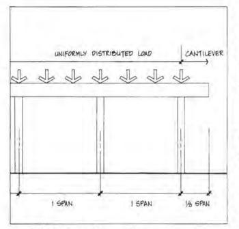
Figure 4.39. Floor Beam with Cantilever Overhang
