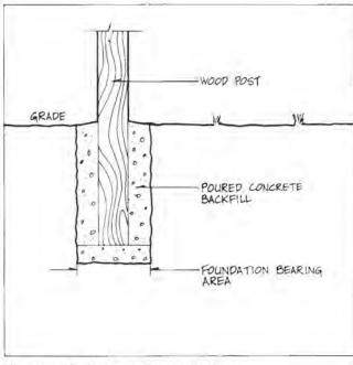
Figure 4.7. Post on Concrete Bearing Pad
