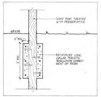
Figure 4.5. Reinforced Concrete Collar
