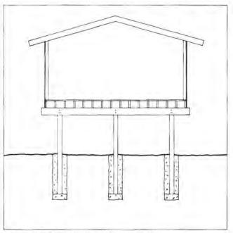
Figure 4.28. Platform Construction
