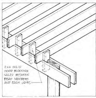
Figure 4.41. Wood Joist Anchors
