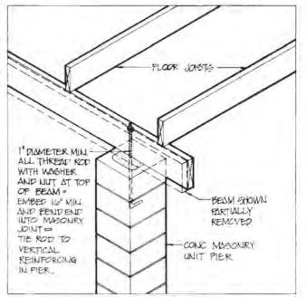
Figure 4.37. Masonry Pier-Bolt Through Beam
