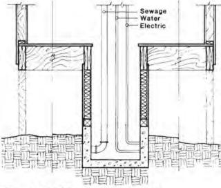
Figure 4.48. Protective Utility Shaft
