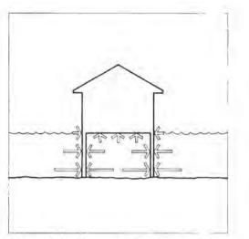
Figure 2.1. Hydrostatic Forces
