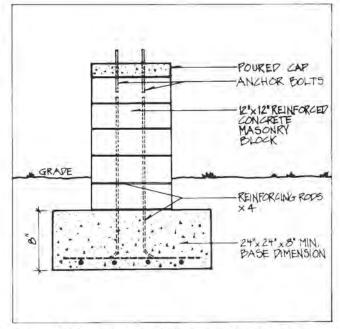
Figure 4.17. Reinforced Concrete Masonry Pier
