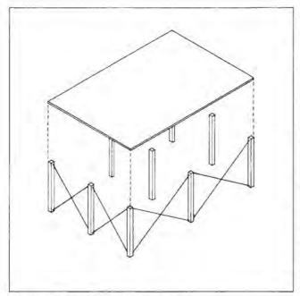
Figure 4.22. Diagonal Bracing
