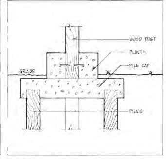
Figure 4.8. Post/Pile Foundation
