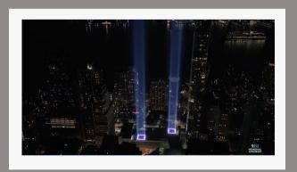
THE TWIN BEAMS ARE SET IN TWO 48-FOOT SQUARES THAT HOLD 88 SEVEN-THOUSAND WATT XENON LIGHTBULBS
