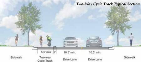
motor traffic by raised medians, on-street parking, or bollards. By separating cyclists from motor traffic, cycle tracks can offer a higher level of security than bike lanes and are attractive to a wider spectrum of the public. http://nacto.org/
